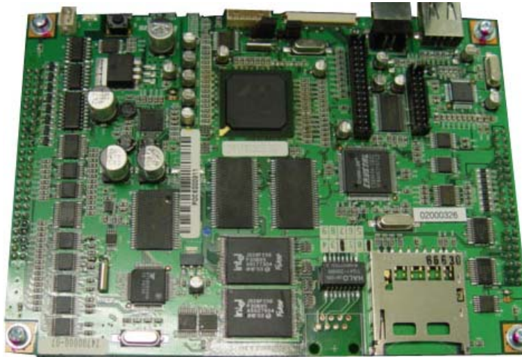
Fig. 3.8 Main Control Board
