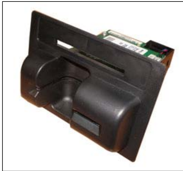
Fig. 3.6 Magnetic Card Reader
