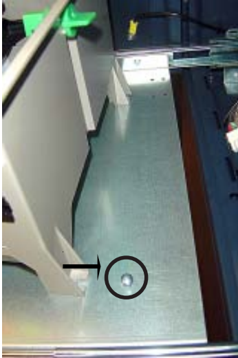
Figure 4. Align slots of dispenser under screws.
