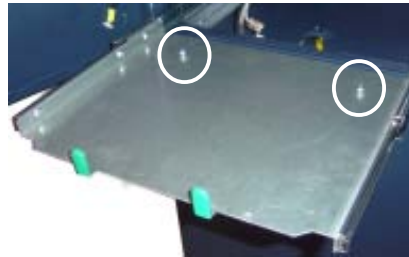
Figure 3. Loosen phillip screws in rear mounting holes.
