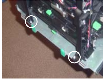
Figure 5. Install front mounting screws.
