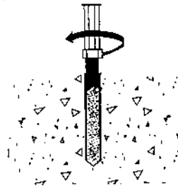
Drive anchor rod into capsule using hammer drill.
