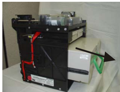
Removing note cassette (TDM-100).
