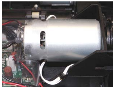
DC drive motor from TDM-1XX modified
