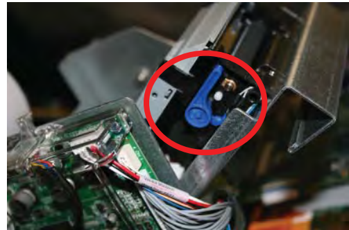
Blue tension lever (correct position).
