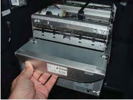
Removing note tray from the dispensing mechanism.
