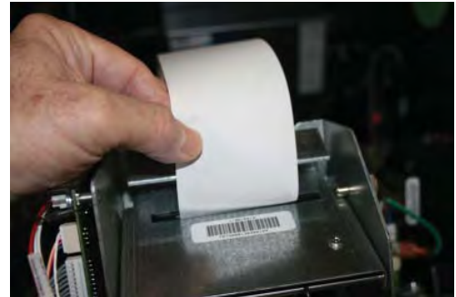
Feed paper into the printer take-up slot.
