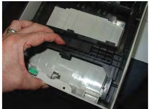
Pull packer plate back before loading notes.
