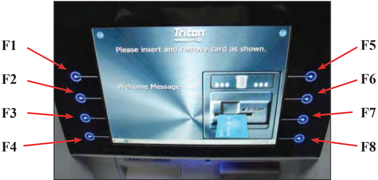
Function key layout on 12.1" screen.
