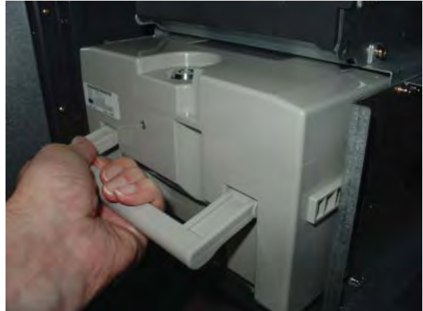
Removing note tray from the dispensing mechanism.
