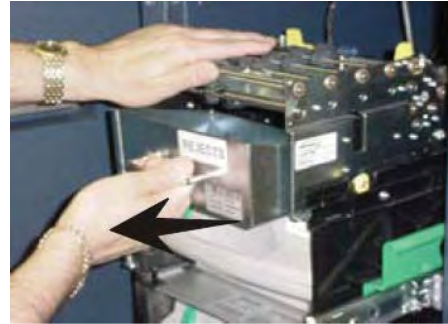
Removing the reject vault
