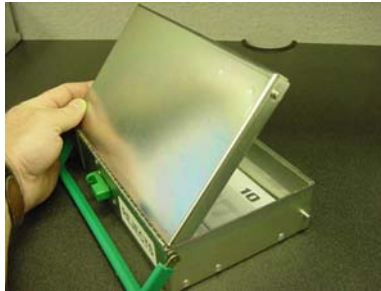
Open reject vault top.
