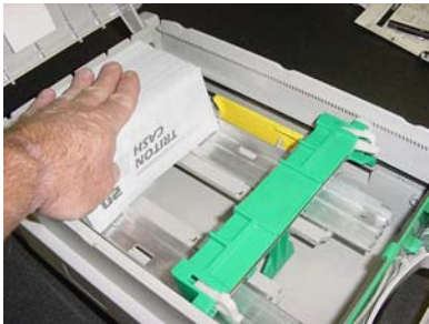
Level the note pile.
