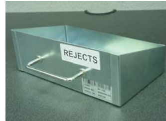
Open (non-lockable) reject vault.
