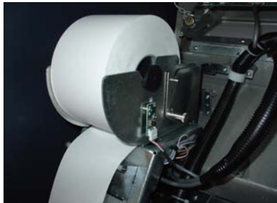
Figure 6-5. Paper on support bracket ready to be loaded into printer. Paper feeds from Bottom .
