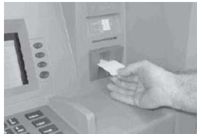
Figure 6-10. Use the cleaning cards on a monthly basis to maintain effective card reader operation.
