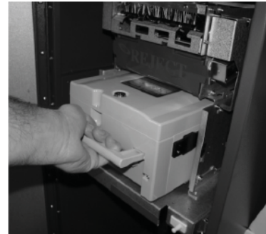
Removing note tray from the dispensing mechanism.
